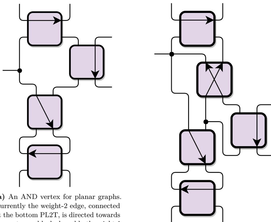
(a) An AND vertex for planar graphs. Currently the weight-2 edge, connected at the bottom PL2T, is directed towards the vertex and locked, and both weight-1 edges are directed away. If the weight-1 edges become directed towards the vertex, the robot can visit the vertex gadget and traverse a loop through all three PL2Ts, locking the weight-1 edges and unlocking the weight-2 edge. The CL2T is a sufficient crossover.
