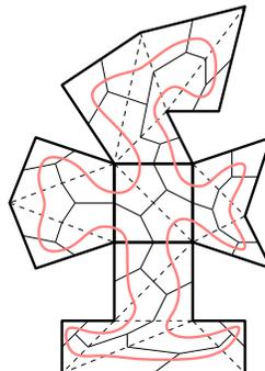
**Fig. 6.** Hamiltonian refinement of five faces in a hypothetical polyhedron, shown here unfolded. Bold lines outline faces. Dashed lines show triangulations and are not cuts. Thin solid lines are cuts. The curved line shows a Hamiltonian cycle induced by the spanning tree of this unfolding.
