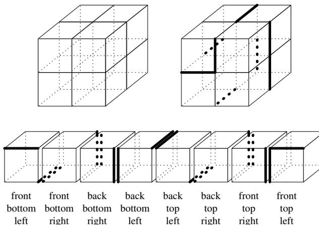
**Fig. 8.** A hinged dissection of a cube into a  $2 \times 2 \times 2$  array of 8 subcubes. This hinged dissection can be used in place of that in Figure 5; every face has (at least) one exposed hinge. Top-left: The dissection. Top-right: The cyclic hinging. Bottom: Unfolded after cutting one hinge. Hinges are drawn bold.
