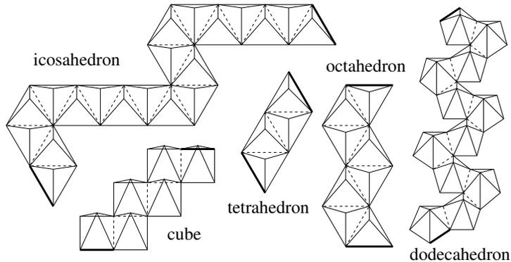
**Fig. 5.** Unfolded exposed cyclic hinged dissections of the platonic solids. The bold lines indicate a pair of edges that are joined by a hinge but have been separated in this figure to permit unfolding. The dashed lines denote all other hinges between pieces. In the unfolding, the bases of all of the pyramid pieces lie on a plane, and the apexes lie above that plane (closer to the viewer).
