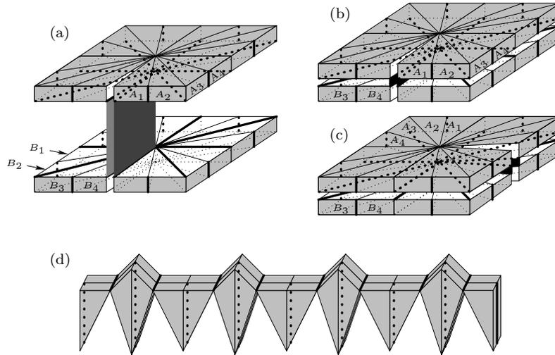
**Fig. 7.** The twister gadget with  $k = 4$ : 32 pieces allowing any between none and three quarter turns. For visual clarity, the two layers are drawn substantially separated in (a) and slightly separated in (b) and (c); in fact they are flush. (d) shows the result of unfolding along the perimeter hinges. (c) shows a refolding that achieves a half turn.
