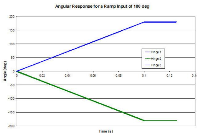
**Fig. 2 Response of accordion origami to a step input of +/- 180 deg**
