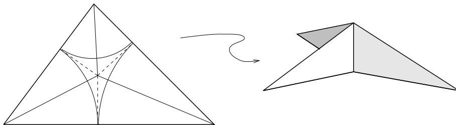
Figure 2: A rabbit ear molecule folds into a three-armed “starfish”.
