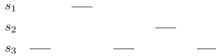
Figure 3-8: Here, the costliest merge is that of either s_1 and s_3 or s_2 and s_3 . This would result in a total cost of 6, assuming unit gap cost. Yet the most expensive merge sequence involves merging s_1 and s_2 first, then merging with s_3 for a total cost of 7.
