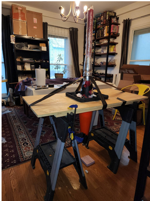
Fig. 5: Scaffold holding the glass handle and ferrule together while the adhesive cures. © Mariel Bass, Erik Demaine, Martin Demaine.
