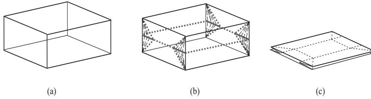
Figure 1: (a) A box; (b) mountain and valley creases are showed by bold grey line segments and bold grey dotted line segments respectively for the final flat folded state, together with long dotted line segments for moving creases; (c) the final flat folded state.
