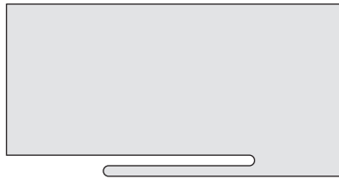
Figure 12. A polygon with two hairpin vertices. All three bottom horizontal segments are collinear. No flips are possible, but this polygon is not convex.
