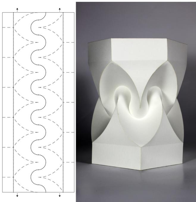
Figure 2: Physical reconstruction of Huffman's model
