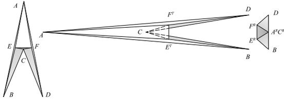
Figure 3: An edge-ununfoldable polyhedron with 6 vertices and 7 faces.
