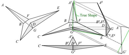
Figure 1: An edge-ununfoldable polyhedron with 7 vertices and 6 faces.
