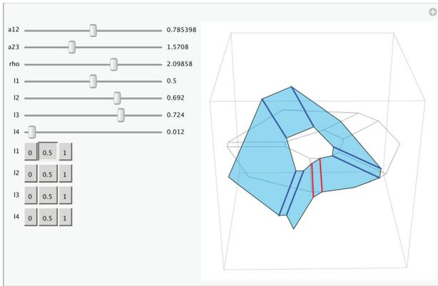
**Fig. 10** Parameterized thick single-vertex construction in Mathematica
