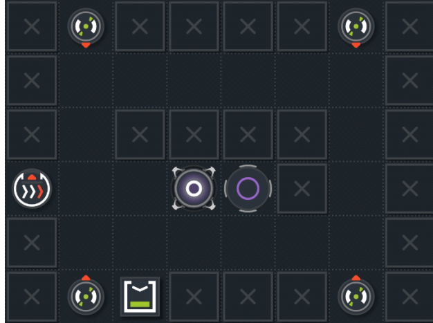
Figure 3.35: A cycle for the mover to deliver binary units. The two objects in the middle are the source and target. If the mover enters at the left as shown, it is pulled into the loop similarly to the fan-in. The turners then keep it moving in a rectangle, and it moves a binary unit from the source to the target on each loop.
