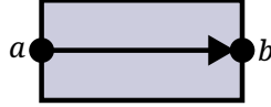
Figure 2-1: The diode gizmo G . L = \{a, b\} , and G is the set generated by the regular expression ([a \rightarrow a] \mid [a \rightarrow b] \mid [b \rightarrow b])^* .
